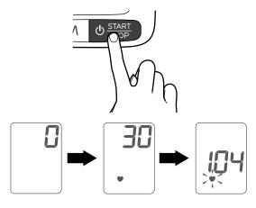
is displayed when a pulse is detected.
